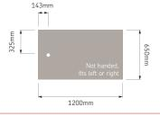
Tray with gravity waste code: 16360W Tray with upward pump waste code: 16361 Tray only code: 16360
