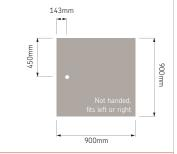
Tray with gravity waste code: 16472W Tray with upward pump waste code: 16473 Tray only code: 16472
