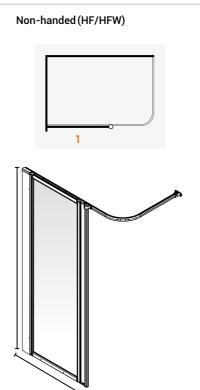
Please note: Compensators are set at mid point giving 14.5mm in and out adjustment on one side. Screen width needs to be less than the length of the tray and provide adequate access for user.
